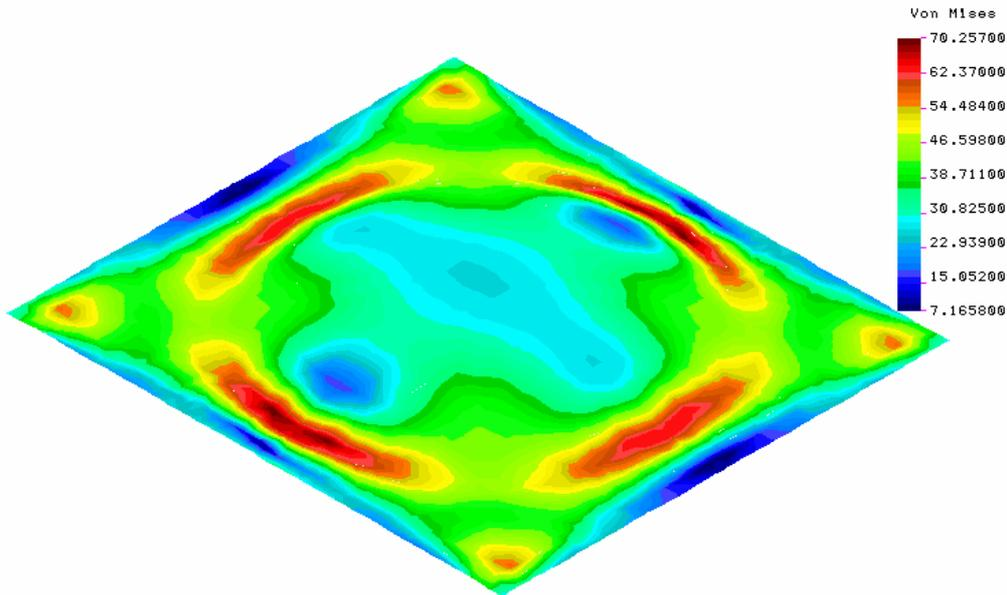
Fig. 12: Von Mises stress field in the sandwich element under wind suction ( $p = 0.049$  mbar)
