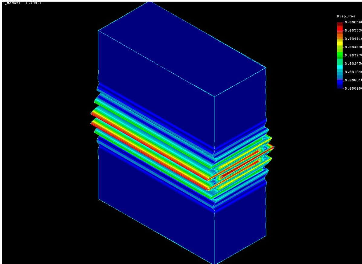
Fig. 9 Wrinkling pattern in a compressed sandwich panel
