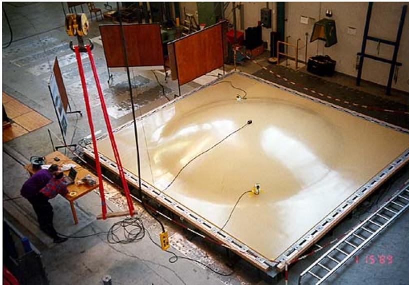
Fig. 6: A photograph of the test plate. The photo shows the plate, the edge connections, and the transducers, which were installed to measure the natural frequency of the plate with the ambient vibration method.
