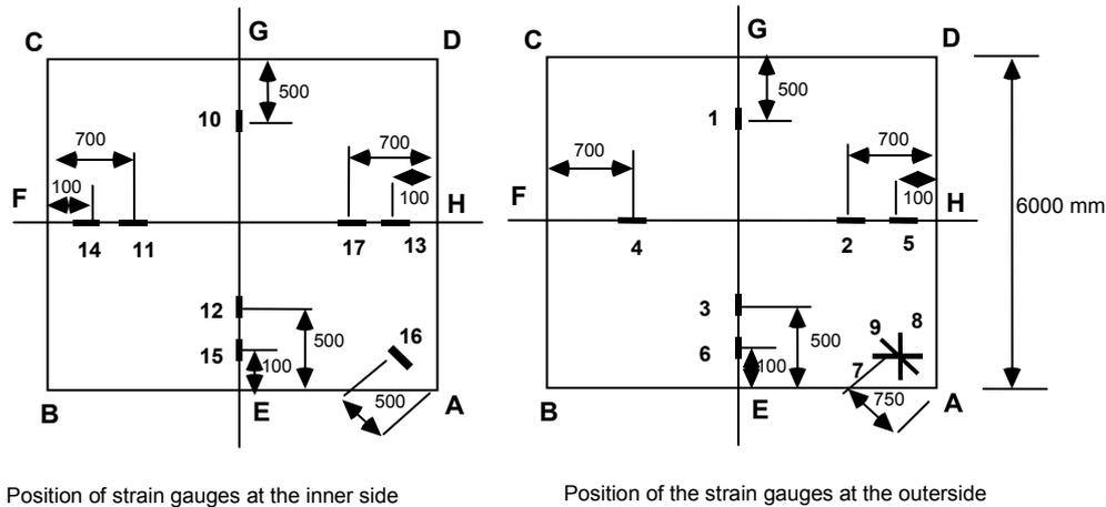
Fig. 7: Arrangement of the strain gauges at the inside and the outside of the test element
