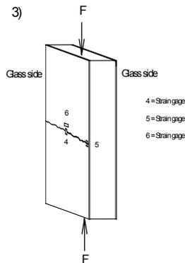
Fig. 4: Wrinkling pattern of sandwich panel No. 6 (PEI core and GFRP facings)
