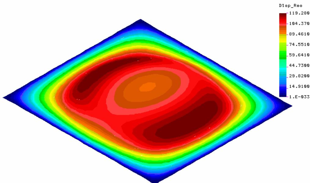
Fig. 11: Resultant displacement field in the sandwich structure under wind suction ( $p = 0.049$  mbar)
