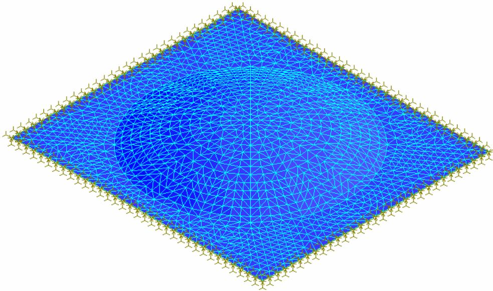
Fig. 10: Finite-Element model of 6.0 m x 6.6 m sandwich element
