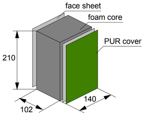
Fig. 2 Overall dimensions of sandwich samples for wrinkling tests
