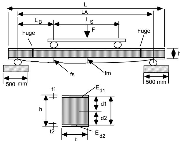
Fig.1: The experimental arrangement and the geometrical parameters in the four points bending tests on sandwich beams
