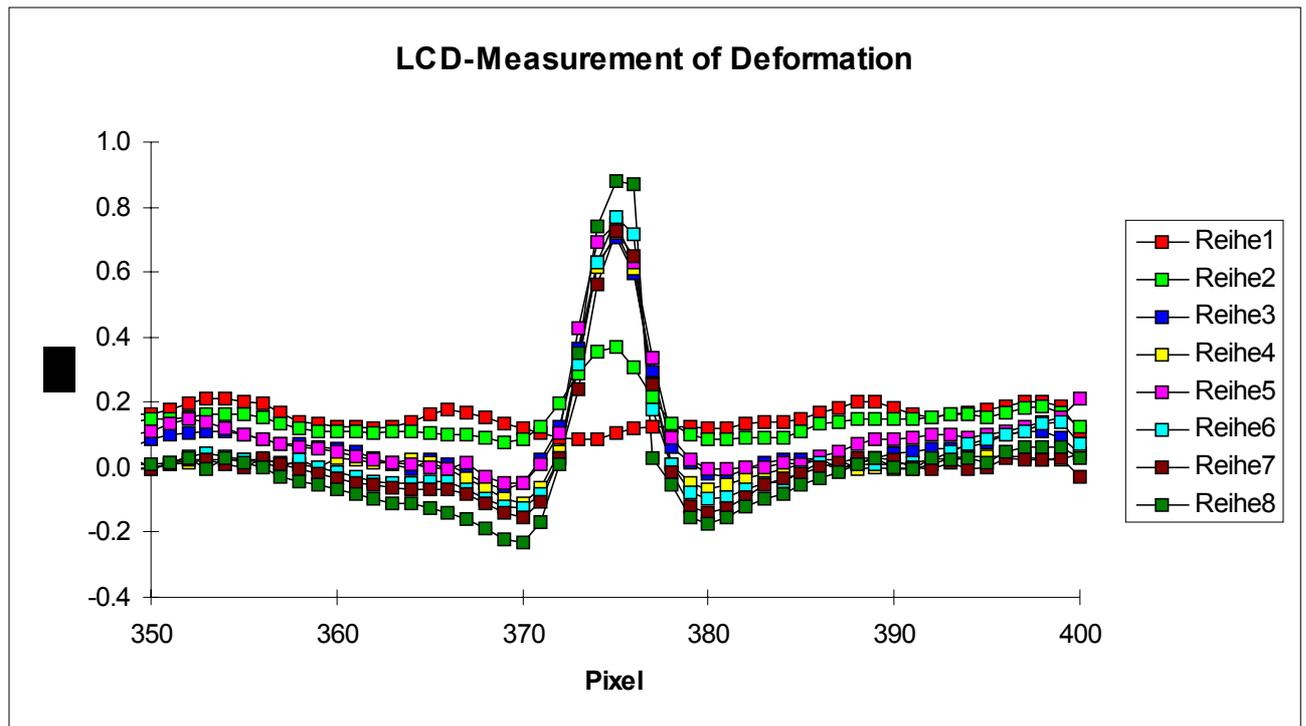
Fig. 5: Lateral deformation profile of the facing of sandwich sample No. 8 under axial compression obtained by the Moiré photographic technique. The Legend including the word "Reihe" designates the sequence of Moiré readings.
