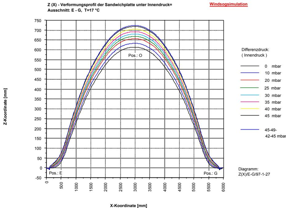
Fig. 8: Undeformed and deformed mid section profile of the sandwich structure in the x direction at various values of wind suction
